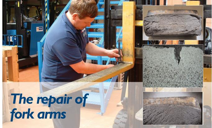
Forming a critical part of a fork lift truck, fork arms are the steel component which physically accepts a load. They are designed, manufactured and tested to accept dynamic, bending and torsional stresses in the truck's day-to-day operation. Abuse, incorrect use or improper maintenance decreases the life of the forks. Because of this, we are often asked by CFTS members, as well as truck users, about the criteria regarding their repair.
